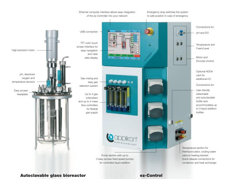
combination of ease of use and sophistication, reducing the time to start-up a process. The system is equipped with the intelligent and powerful process controller: easy and intuitive to operate, such that the user manual might not be needed.
